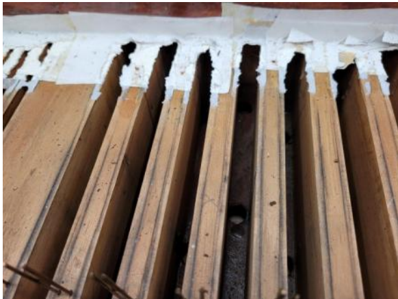
The top of the Table— splits screwed, pegged and glued
