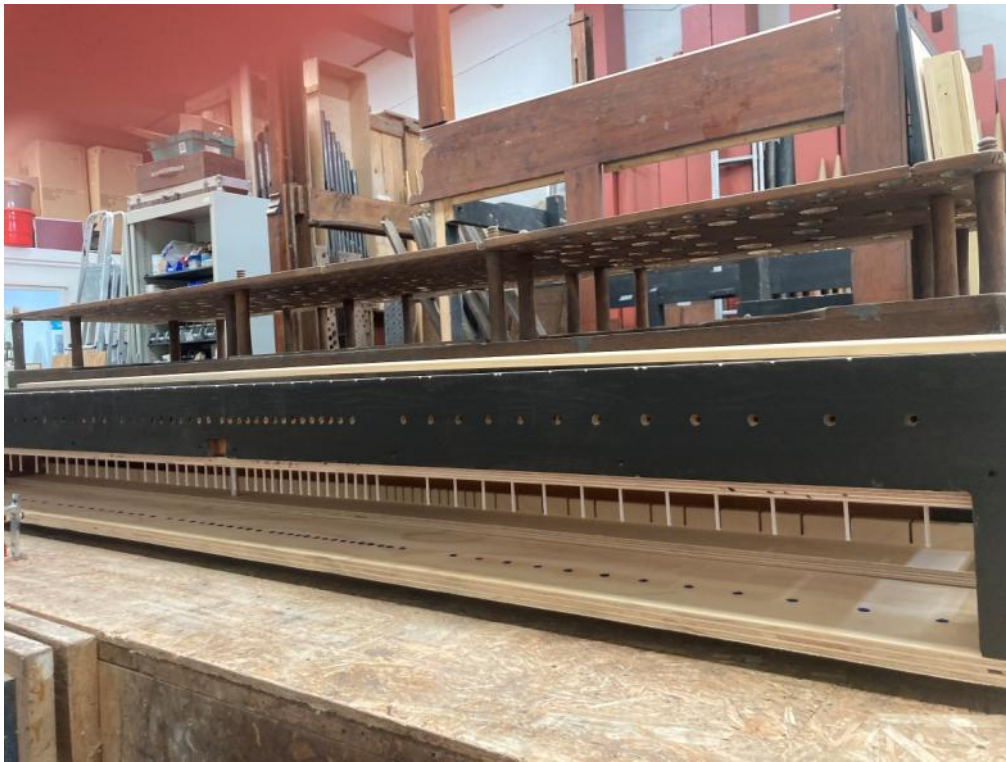
11th Sept 2024 The Swell Soundboard with new Bottom Board, Pallet Board and Pallet Guide Pegs with the old Upper Boards and Pipe Rack placed on top.
