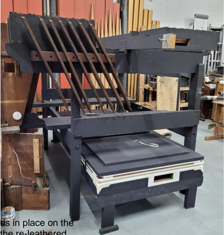
Great Soundboard with the new magnets mounted in the new pallet box underneath
