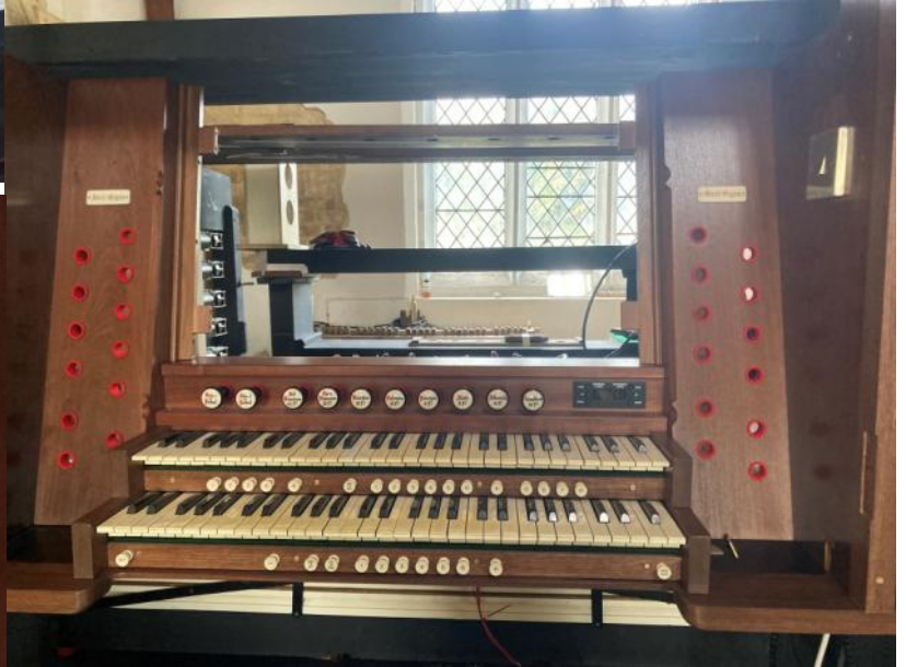
6 th March: stop jambs, pedal stop knobs and Great slider motors installed
