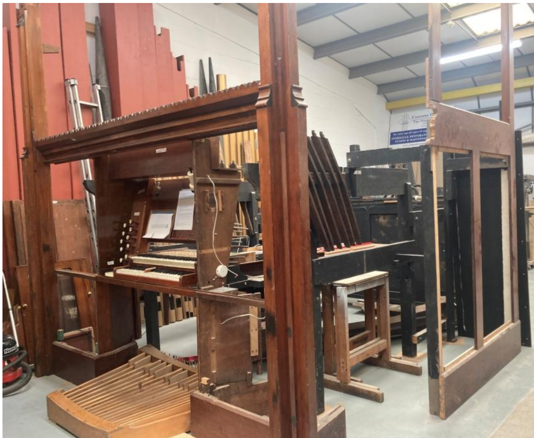
The organ frame and part of the case being assembled with new Keyboards and Pedalboard.
