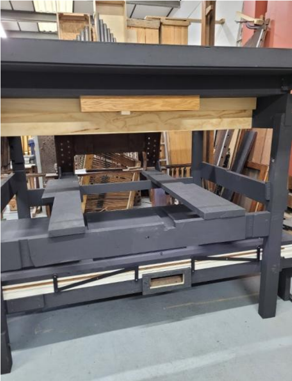
Back of the Swell Soundboard with the new pallet box for the magnets below and the re-leathered bellows at the bottom,
